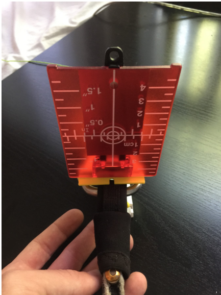
6. Attach Laser Target Using Magnet.
