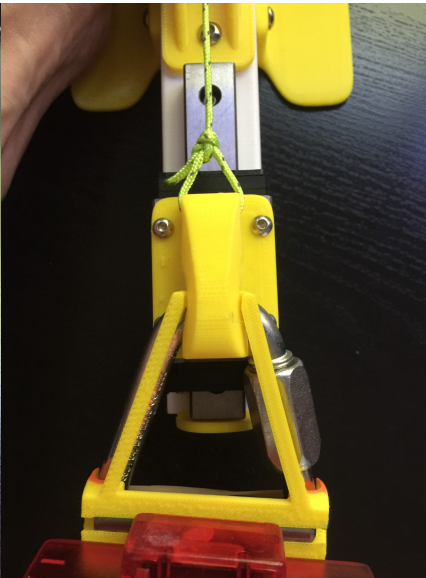
7. When Measuring Do Not Bottom Out to ensure proper Loading
