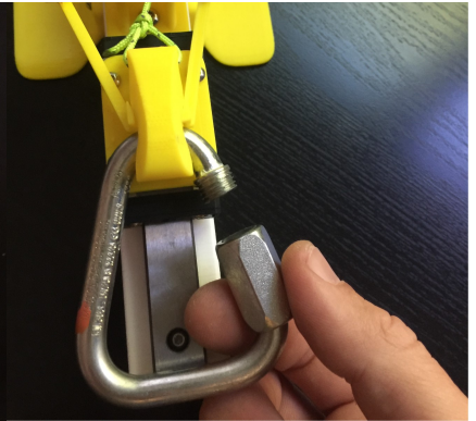
3. Carefully, Flip Up Target Mount Open Maillon for Riser.
